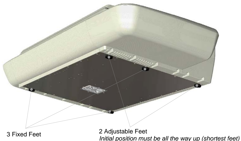
Fig. 11-1, Physical Placement of the Scanner
